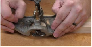
Many tenons are centered on the end of a workpiece. To maintain this balance, what you do to one face you must also do to the opposite face. Keep this in mind if you are using the router plane to adjust the fit of a slightly oversized tenon. Remove only half of the excess thickness from a single face.
