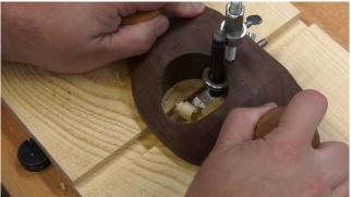
for this purpose. You might set such a stop to the full optimal depth, then work to it through smaller adjustments.
