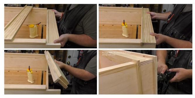
The secret compartment is built into the top of the bookcase and made to look like a moulding. This process provides a lesson in cutting parts to fit rather than to the sizes on a cut list.
