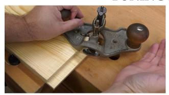
A rabbet is worked much like a dado, beginning with severing the fibers along the inner shoulder with a knife.
