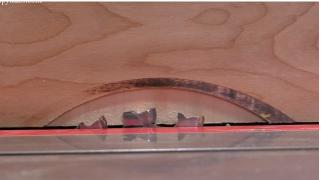
Dado sets create momentum that may lift the workpiece, especially at the beginning and end of the cut. Stock that's not perfectly flat can also lead to inconsistent joinery. Push blocks with nice, grippy bottoms will make it a lot easier to apply pressure in two directions- downward and against the fence. You may even make a second pass just to be sure the rabbet was cut to a consistent width and depth along the entire edge.
