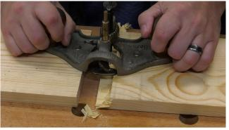
You may also support the overhanging portion of the plane's sole with another workpiece of equal thickness. Two identical rabbets could also be cut at the same time if they are placed end-to-end. This will make it more difficult to take circular bites, forcing you to cut the fibers as you would a dado. But the process will achieve good results if you are able to secure your workpieces to the bench to prevent movement.
