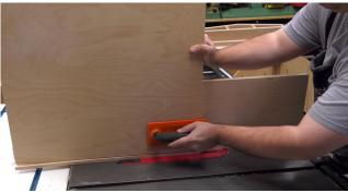
the two layers together so you may need to add shims or tape between them to square the fence panel to the top of your saw.
