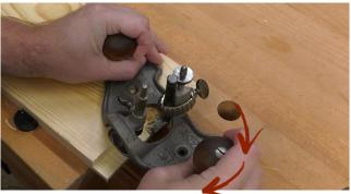
the rest of the body extends off the end of the board. That handle becomes a pivot point as your other hand to turns the router toward your body, moving the cutter into the material. Repeat this process, taking bites all along the rabbet while keeping half the sole flat on the face of the board. This will leave a lot of shredded fibers behind which may then be cleaned up with a final, straight pass along the entire rabbet.
