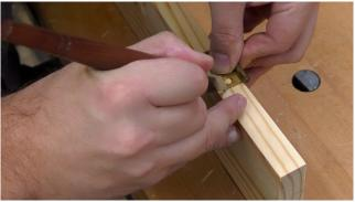
keep the sole flat on the edge of the workpiece. If you have difficulty preventing the plane from tipping you may clamp a second board to your workpiece to temporarily make it "thicker" and better support the plane.
