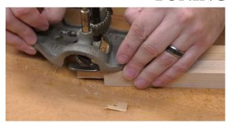
A tenon is just a series of rabbets, and the process of tuning one with a router plane is not too different. One hand holds the sole of the plane flat on the board's face while the other hand twists the plane, cutting into the wood in a circular motion.
