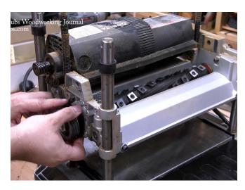
es on even the toughest grain. It is far easier to rotate the cutters on a helical head than it is to change conventional knives, and each cutter has four carbide edges which last many, many times longer than high speed steel.
