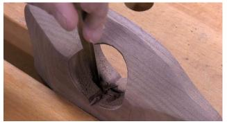
Perhaps the most difficult part of the build is cutting the groove that holds the shaft of the cutter, and the mortise that accepts the eye-bolt which secures the cutter in place.
