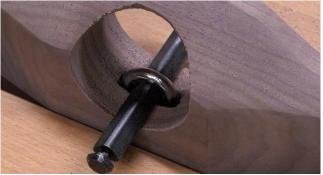
The mortise must be cut across the groove, and it need not be as precise. Still, it was tricky because the shape of the plane's body interfered with my chisel. The mortise is cut only part way into the body and a hole is counter-bored from the opposite side. The shaft of the eye bolt slips into the hole and as a nut is tightened, the head of the bolt is drawn into the mortise, securing the cutter in it's groove.
