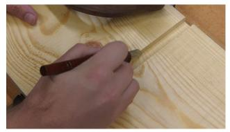
If a board is cupped, a dado is likely to be shallower in its center than it is at its ends. A bow along a board's length may cause a similar affect when a groove is formed. To correct this problem, set the router plane's cutter to the depth you wish for the entire groove.
