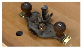
A router plane may be the fastest way to cut a mortise for a hinge.
