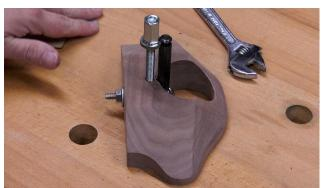
Another challenge presented itself when I installed the threaded post behind the cutter. This must be perfectly parallel to the cutter's shaft where it is held in place with epoxy.
